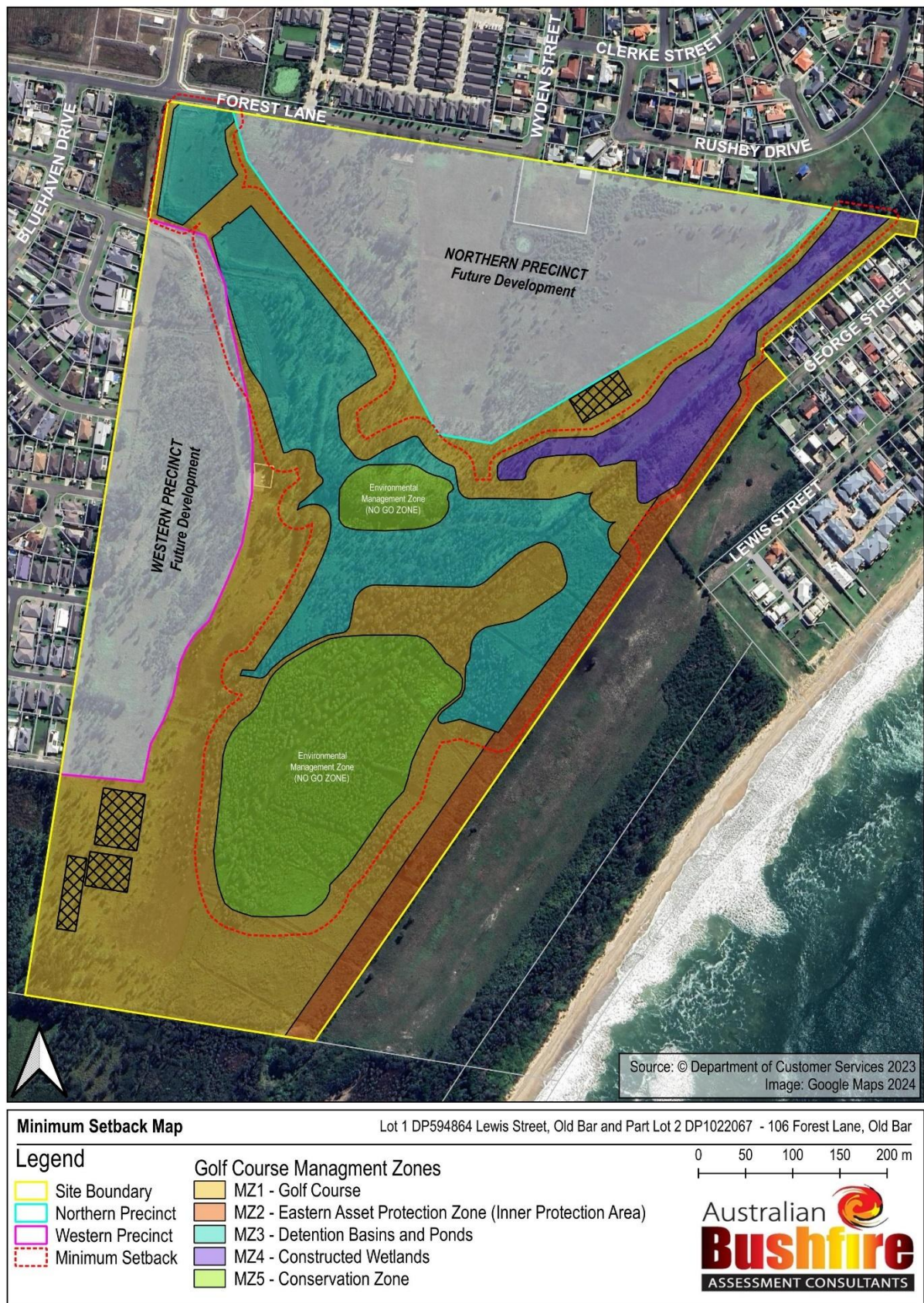
Figure 5.1: Minimum separation distances relative to proposed vegetation management zones (PBP Table A1.12.3, FDI 80, <29kW/m 2 )
